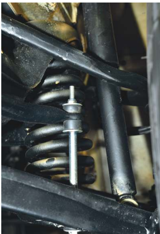
Left Every aspect of Bim's 300 SL is utterly spotless, including its chassis and suspension equipment, which has been treated to cleaning, shot-blasting, powdercoating and full wax protection
